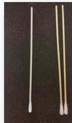
Left: synthetic swabs with plastic handles (use) Right: cotton swabs with wooden handles (do not use)
